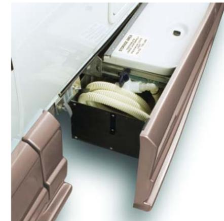
The macerator sewage pump on 210 and RS models chops up any solids and tissue and ejects the entire contents through a convenient 1/4" hose. No mess, no fuss.
