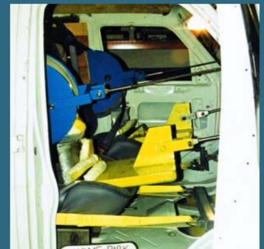
These 2 photos depict simultaneous seat belt testing and seating system testing. Seat belt testing confirms proper seat belt location and minimizes the possibility of anchorage failures. Seating system testing verifies the integrity of the seats, their attachments, mounting hardware and installation.
