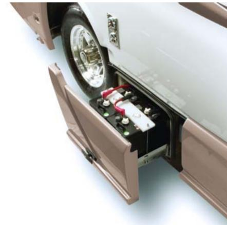
Our 210 models feature an optional auxiliary battery system with two lead acid deep cycle 6V batteries with 220 total amp hours located in a convenient slide-out drawer.
