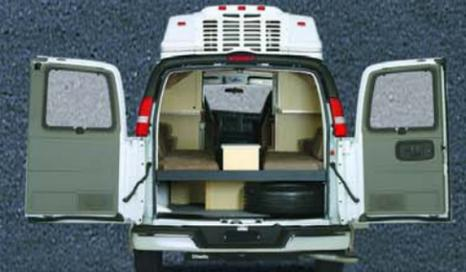
Dual rear doors allow for easy rear loading and swing a full 180° on 170 and 190 models and 270° on RS models.
