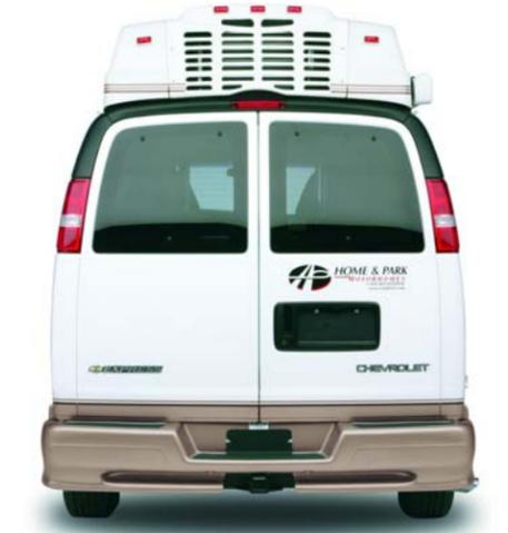
A 'Dometic' heat pump (air conditioner & heater) built into a recess in the roof cools the interior while maintaining Chevy based Roadtrek's aerodynamic shape and sleek roofline. In many restricted communities, vehicles with roof mounted air conditioning units are not permitted. Our recessed heat pump allows our Chevy based motorhome to be perceived as just a van and in most cases is permitted to park where many other motorhomes are not.
