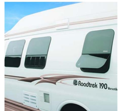
Frameless awning windows are better looking, reduce wind noise, improve aerodynamics, and provide superior air circulation even during foul weather. Their larger size provides a better view from inside. The Integrated Venting System (170 and 190 models) provides inconspicuous ventilation of the refrigerator.
