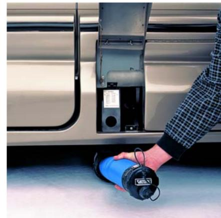
Easily accessible, our patented built-in sewage hose system on 170 and 190 models provides a permanently attached sewage hose that eliminates messy handling and storage. The wastewater tank releases and the fresh water tank drain are adjacent.
