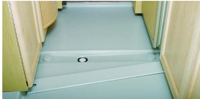
A removable cover in Chevy based Roadtreks reveals a trough with a drain that spans the lowered floor and prevents water from leaving the shower area.
